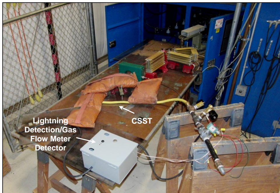
Figure 7 – Lightning Detection/Gas Flow Meter Detector Unit Test Setup
