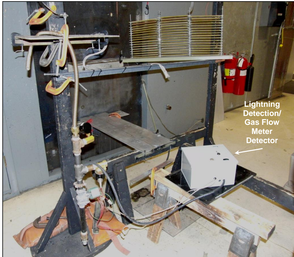
Figure 5 – Lightning Detection/Gas Flow Meter Detector Test Setup
